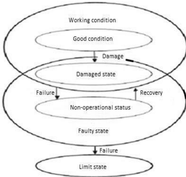
Figure 1.2 - Diagram of the Technical State and Events During the Operation of CTS
