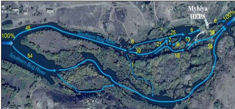
Fig. 5. Distribution of flow over the Southern Bug River water system in the region of Myhiya village in the low water period of the year. Figures on the diagram – the share of flow on a separate site in% of the total river flow (water consumption 43 m 3 /s). According to the materials of full-scale shooting 18.07.2017
